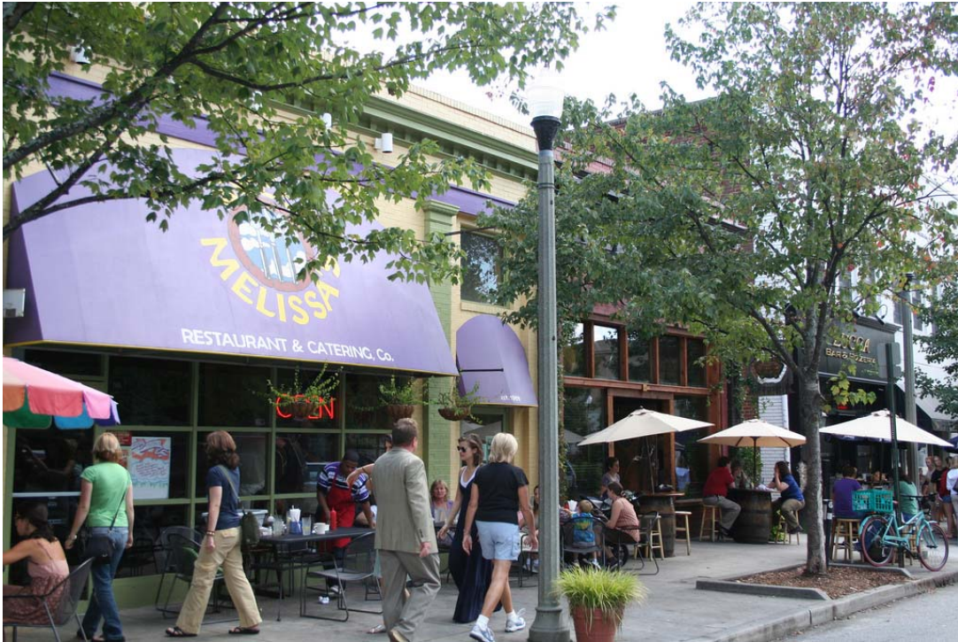
Figure 130-3 Collection of buildings that employs vertical and horizontal changes, cornice variations, and a range of window styles. Note that most of the ground floor openings have lots of glass, which is desirable.
