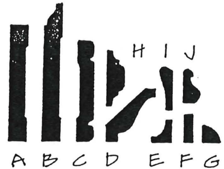
Types of molding shapes. A) base; B) base with integral ogee cap; C) chair rail; D) crown; E) cove; F) lattice; G) quarter round; H) astragal; I) picture; J) base cap.
